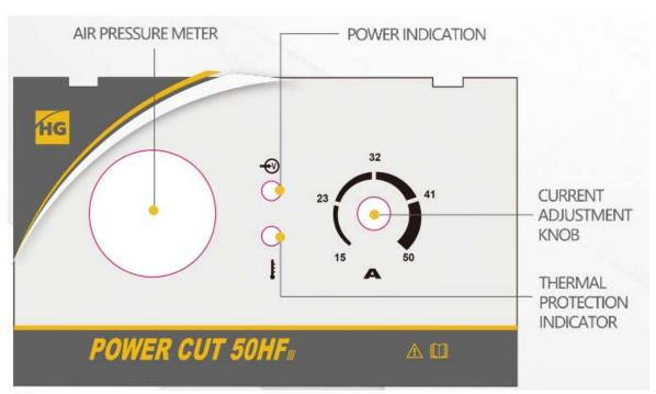
Simple & Easy; Easy set up and use; . Hook up the compressed air, grab the torch and start cutting.
